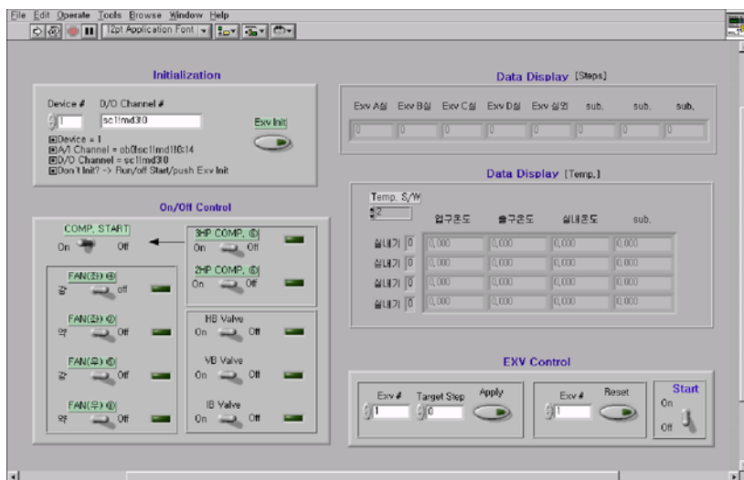
Fig. 4-4 Main display for control system
